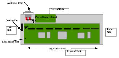
Figure 3.9.1b: Magnum QS5116, Top View with Chassis Cover
